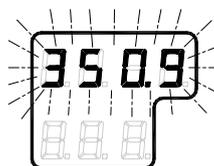
An alarm code for an active error may be recalled by pressing the **DISP** button until the alarm display is shown. It is possible to recall any alarm code in the LCD for as long as the alarm situation is present.
