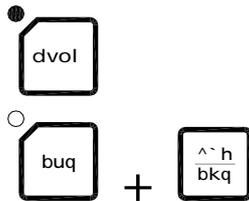
By pressing the **GYRO** or the **EXT** and the **ACK/ENT** buttons simultaneously, the GC80/GC85 will toggle between using the gyrocompass or an external sensor as active sensor.
