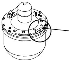
**6** Fasten the screw on the plug holder on the defective Sensitive element.
