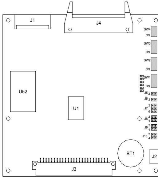
**DIP switch settings on SCC board**
