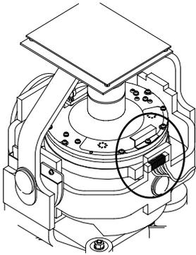
**8** Tilt the Horizontal ring to the side where the plug is located, and carefully put the sensitive element into the ring.
