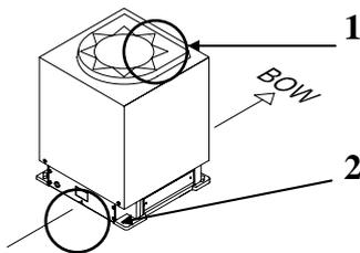
**1** Locate the compass on or parallel to the vessel's horizontal centerline, with the bow indication on the top of the case pointing towards the vessel's bow.
