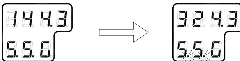
Normal compass operation is resumed by opening the closed potential free contact. The function is indicated by the same acoustic alarm, and the flashing dots returns to fixed illuminated dots.
