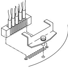
**3** Loosen the screw on the plug-holder on the Sensitive element, and disconnect the plug.
