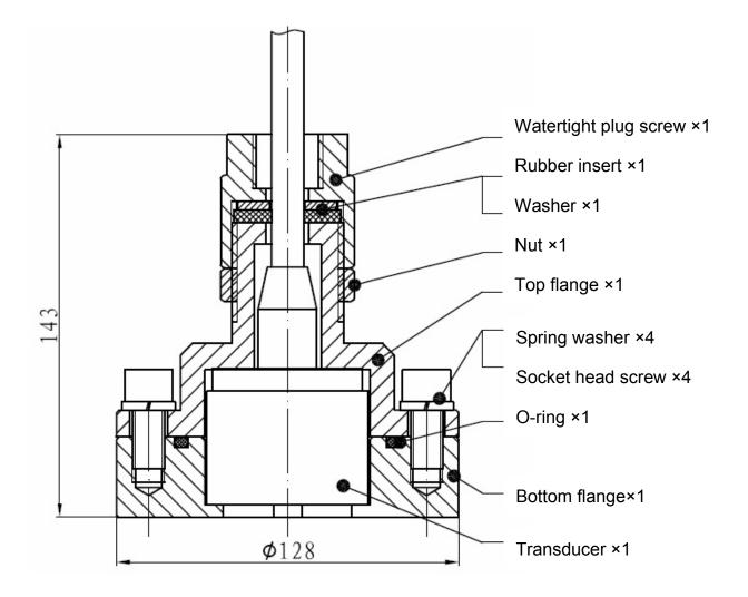
Note, the hole dimension is suggested to  $\phi$ 130mm
