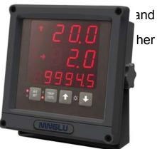
Press TRIP/ TOTL key to switch between trip distance and total distance.
