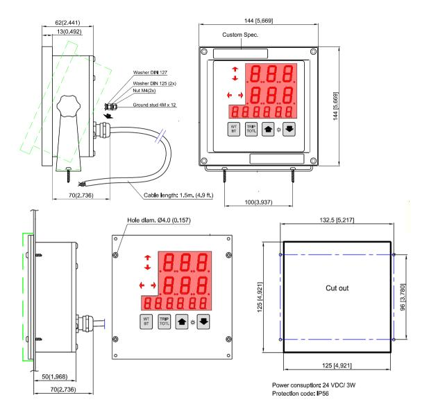
The unit can be mounted in panel, table, wall or ceiling.
