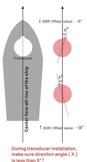
During installation, transducer diameter line through the transducer hump should on the center fore-aft line of the ship. If not, the direction need to be calibrated as showed on the left picture.c-a=GPS speed , and "
