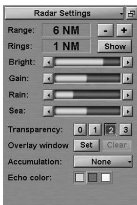
In “Radar Settings” display which will open up, set the range scale. To do this, use the buttons to the right of **Range** input window.
