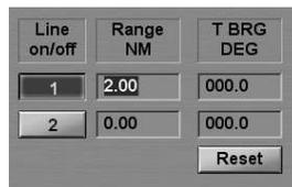
By rolling the mouse, set the required value of distance from the centre of the own ship mark, or enter it from the keyboard. Press the left mouse button. The index line will be set at the specified distance.
