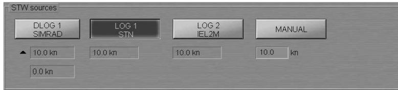
**STW sources** group is designed for selection a source of speed through the water. The group shows all the connected speed through the water sensors.
