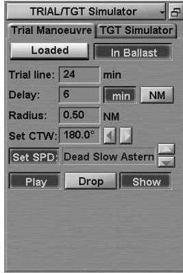
By rolling the trackball horizontally, set the next course. Roll the trackball vertically to set the delay time before the start of the turn. The expected ship motion time is shown dynamically on the ECDIS task screen. The Chart panel displays the own ship motion line with parameters of the intended manoeuvre and the targets' motion lines changed to assume the value set in Trial line box.
