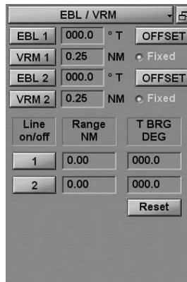
Press the button with index line number. Position the free cursor in the Range input field and press the left mouse button.
