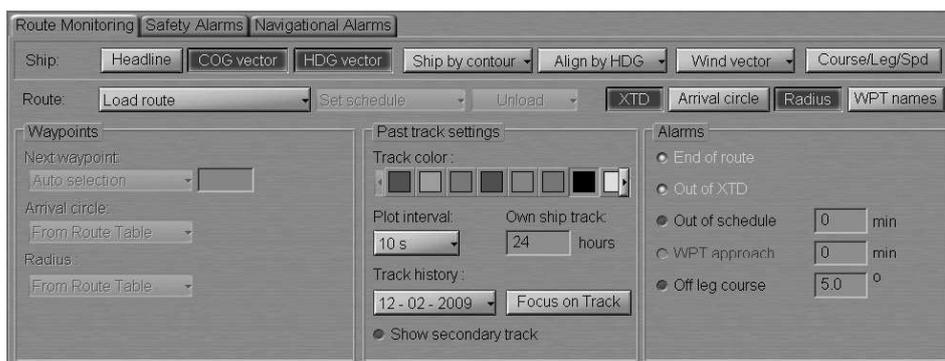
Route group enables loading and unloading of monitored routes and a schedule by using the following buttons:
