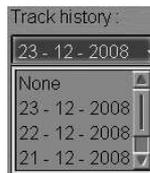
In the list, which will open up, select the date of the track required to be displayed, and press the left trackball/mouse button. The selected date track is displayed on the Chart panel.
