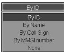
In the list, which will open up, select the necessary identifier or None to declutter the Chart panel. Press the left trackball/mouse button. Targets will be displayed on the Chart panel with the selected identifier, and its name will be shown on the button.
