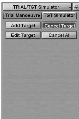
Position the acquisition marker which will appear on the PPI, on the simulator target, which should be deleted.
