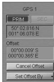
To monitor parameters of the EPFS used for the primary positioning system, press the button with the name of the set display in the Display Panel window of the Control panel.
