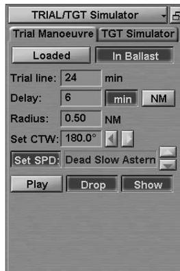
2. The ECDIS task has an alternative mode for entering the intended manoeuvre parameters by using the trackball.
