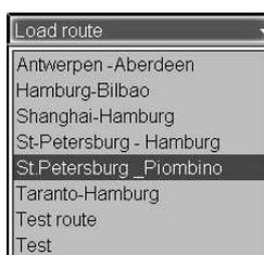
Select the required route and press the left trackball/mouse button. The selected route will be loaded for sailing on the Chart panel, and its name will be shown on the button.
