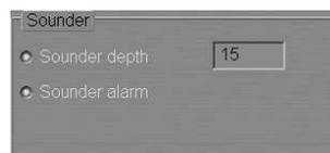
Use **Sounder depth** line to enter the safety depth value from the echo sounder. Check the activated **Sounder depth** checkbox for turning on the alarm generation as a depth smaller than the set one is detected.
