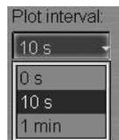
In the list, which will open up, select the track plot interval and press the left trackball/mouse button.
