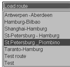
Select the required route and press the left trackball/mouse button. The selected route will be loaded for sailing in the Chart panel, and its name will be displayed on the button. The route loaded for sailing will be shown in red colour.
