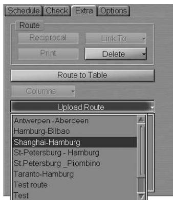
Select the route required to be transmitted and press the left trackball/mouse button. The route will be passed to the external device.
