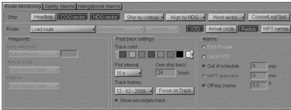
To turn on/off the display of own ship and its motion parameters, press the following buttons in the Ship group:
