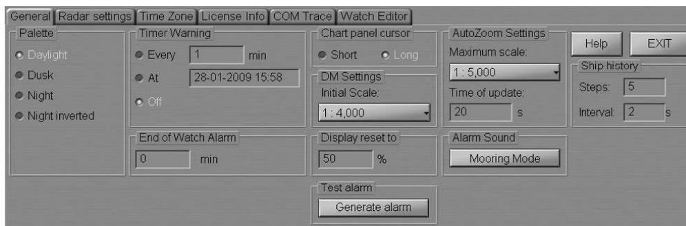
In DM Settings group from the drop-down list select the scale, which will be set on the “Dual” panel as the Docking Mode is turned on.
