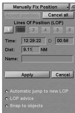
Enter the distance to the object in Dist input box by using the trackball/mouse or keyboard. Press the left trackball/mouse button.
