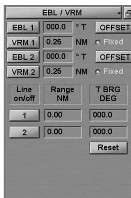
To display the first EBL/VRM pair on the ECDIS task Chart panel, press **EBL 1** and **VRM 1** buttons respectively.
