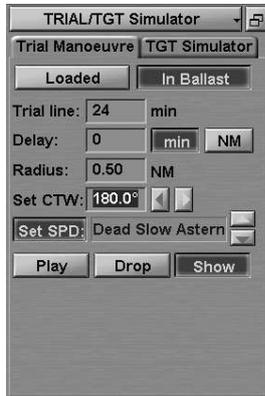
Set the required next course by rolling the trackball/mouse, or enter it from the keyboard. Press the left trackball/mouse button.
