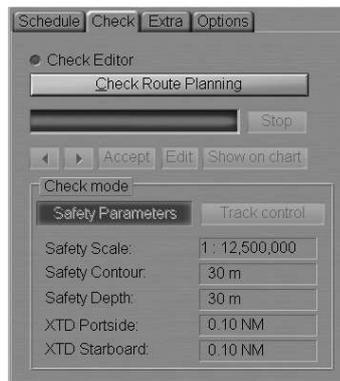
“Check” page serves for checking the generated route for the dangers to navigation. The page contains the following elements:
