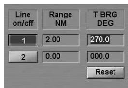
By rolling mouse, set the required value of the index line bearing or enter it from the keyboard. Press the left mouse button. The index line will be set in the specified direction.
