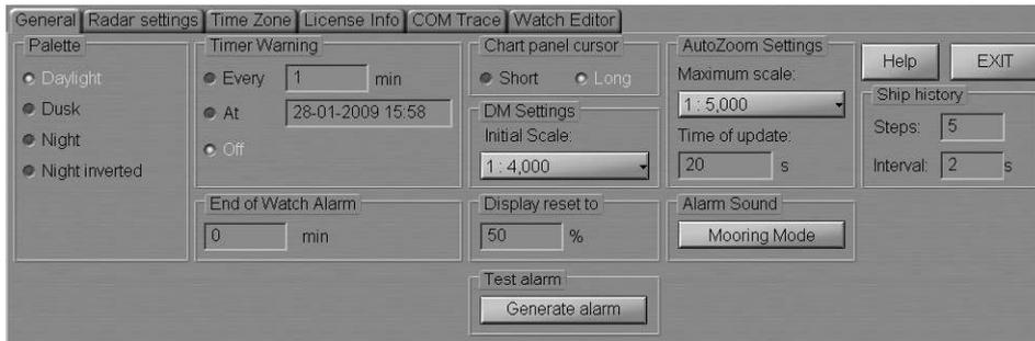
In **AutoZoom Settings** group from the drop-down list, select the maximum scale as the ship is passing the current WPT on “Dual” panel. In **Time of update** input window set the DTW analysis interval.
