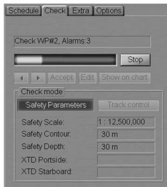
The check process is shown in the display window. After the end of check, “Check” page will display a message about detected dangers or about no dangers having been found.
