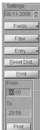
Use **From** and **To** input boxes to set the time interval for the printout of the electronic system logbook events, and press **Print** button.
