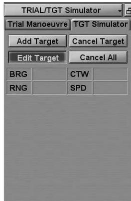
Position the acquisition marker which will appear on the PPI, on the simulator target whose motion vector should be edited.
