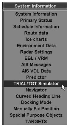
In the list, which will open up, select TRIAL/TGT Simulator line and press the left trackball/mouse button.
