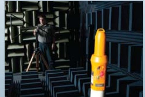
RF Anechoic testing chamber
