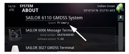
If you have an Alarm Panel in the system, the primary and duplicated systems will appear in the Alarm Panel as Inm-C 1 and Inm-C 2 respectively.
