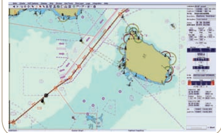
Track control with Anschütz autopilot and ECDIS
